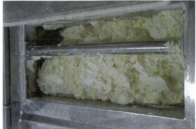
Dry and wet conching of white chocolate in the CHOCO EASY ® process
