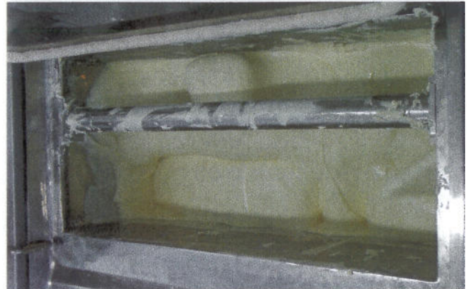
Dry and wet conching of white chocolate in the CHOCO EASY ® process
